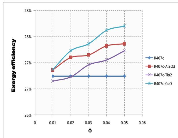
Figure: 5 Variation of Exergy Efficiency with volume fraction ( $\phi$ ) of Vapour Compression Refrigeration System with R407c using different nano particles [25]
