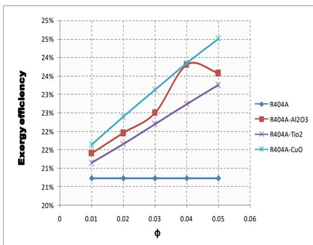
Figure: 6 Variation of Exergy Efficiency with volume fraction ( $\phi$ ) of Vapour Compression Refrigeration System with R404A using different nano particles [25]
